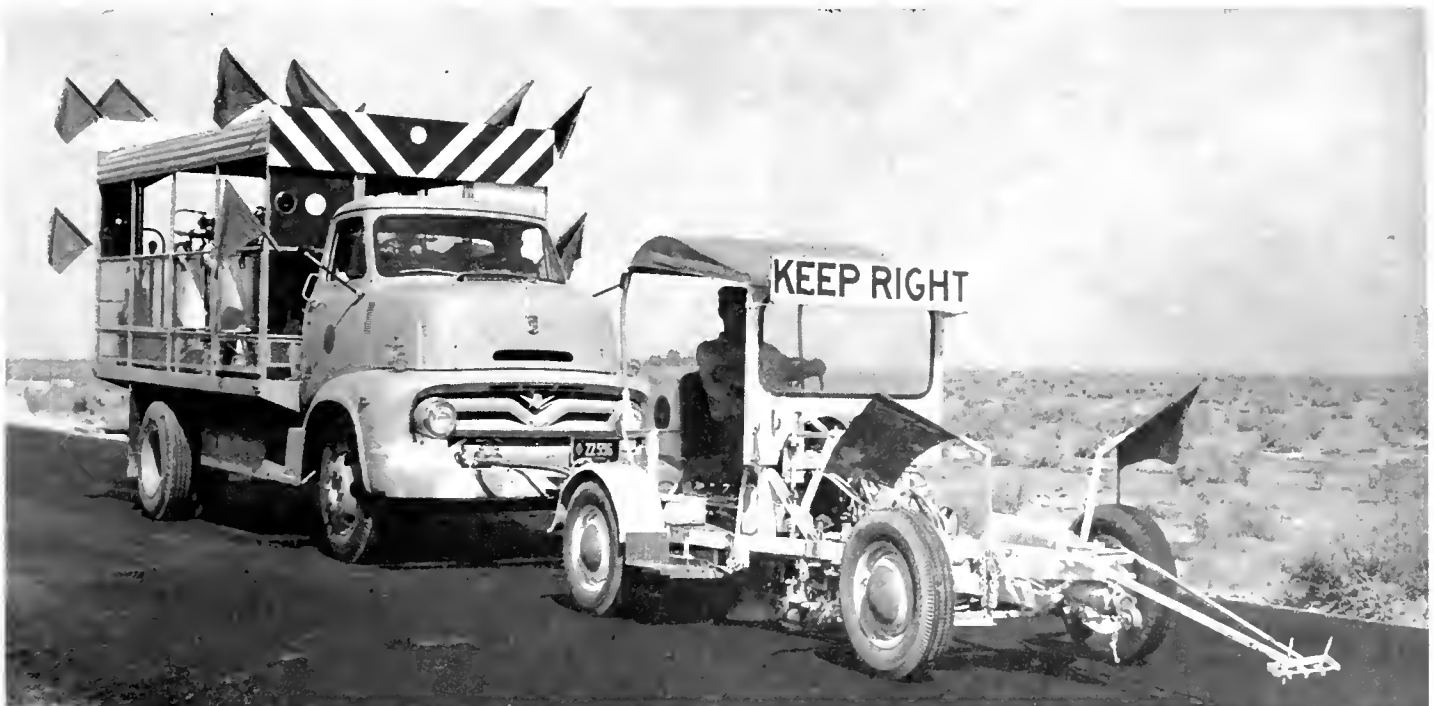
Modern traffic line marker with "mother" truck
